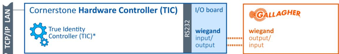
With the addition of a Cornerstone Hardware Controller Cornerstone (TIC), Cornerstone can be configured to communicate with a Gallagher system via a Wiegand connection. The Hardware Controller can also be used to control door strikes and communicate via a Wiegand connection to card readers and other hardware devices.
